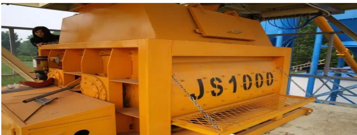
**Figure 2. Central mixing plant**
